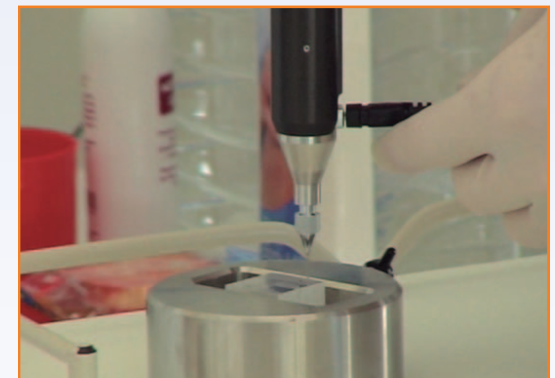
Figure 4: Calibration on PMMA after each measurement in patients
